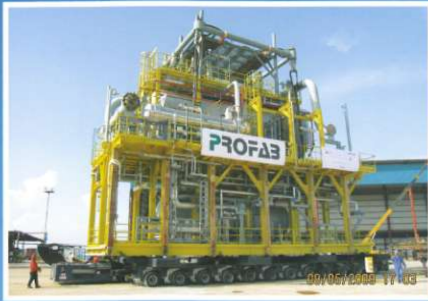
Load-in of 1 unit Glycol Contractor to barge by ro-ro system. Dim. 8m x 8m x 17m (92 Tons).
