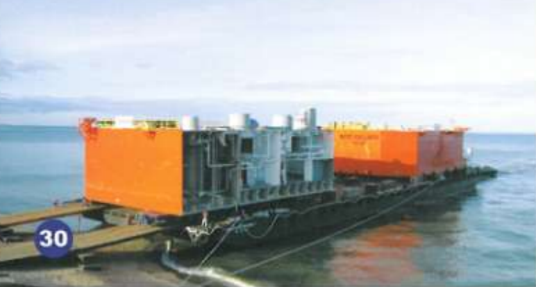
Another successful operation with 2 units Block loaded. Dim. 26.5m x 21.5m x 7.6m (491 Tons) each.
