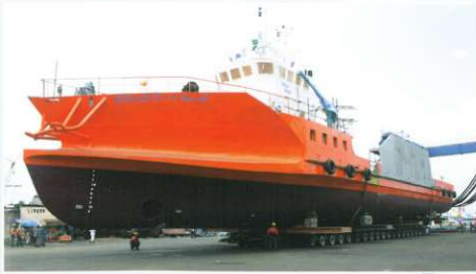
Jacking and shifting of Boat within shipyard. Dim. 55m x 10m x 10m (350 Tons).
