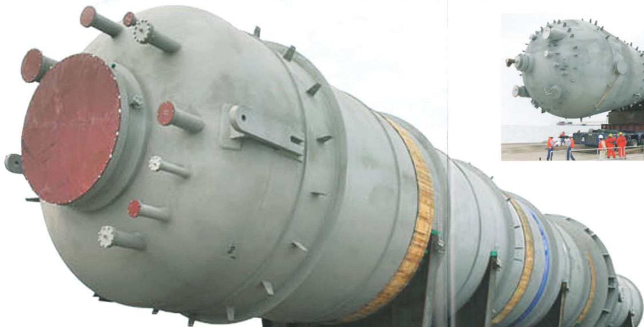
Discharging Purge Bin from barge. Dim. 46.89m x 7.10m x 7.22m (199.5 Tons).
