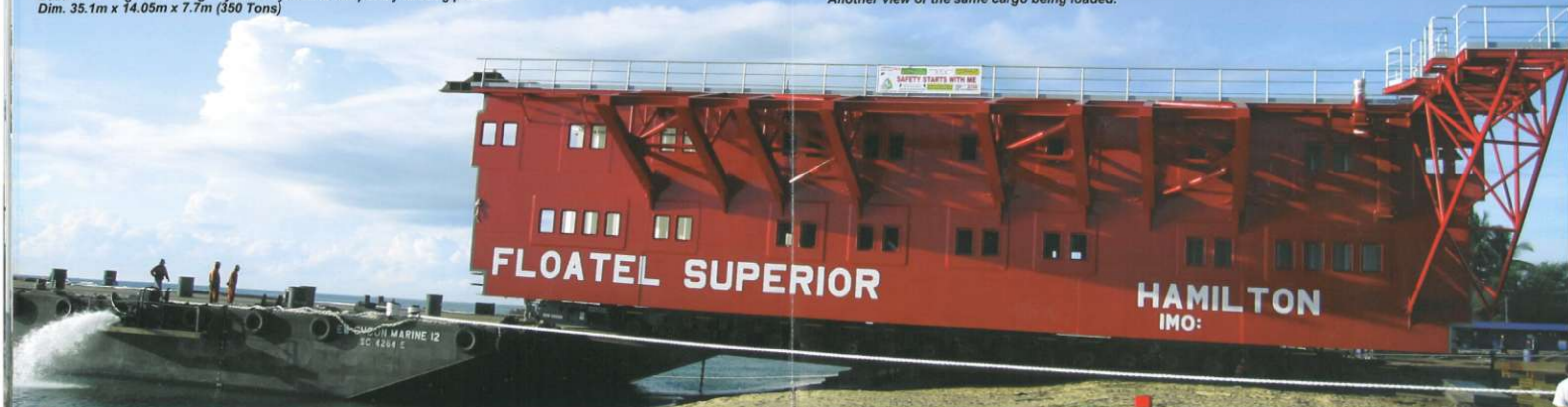
Loading another cargo to barge via ro-ro operation. Dim. 35.1m x 24.7m x 7.7m (785 Tons)
