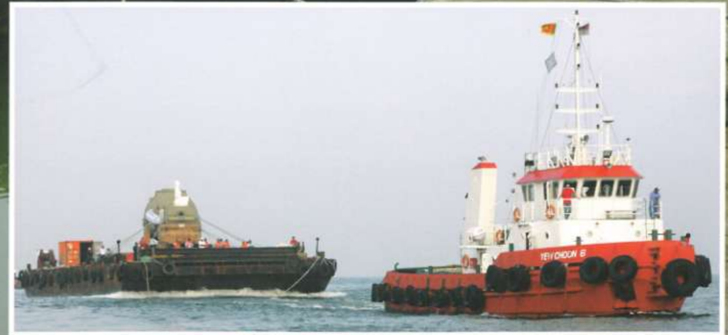
Heavy-duty deck barge with seawater ballasting capability, most suitable for ro-ro operations.
