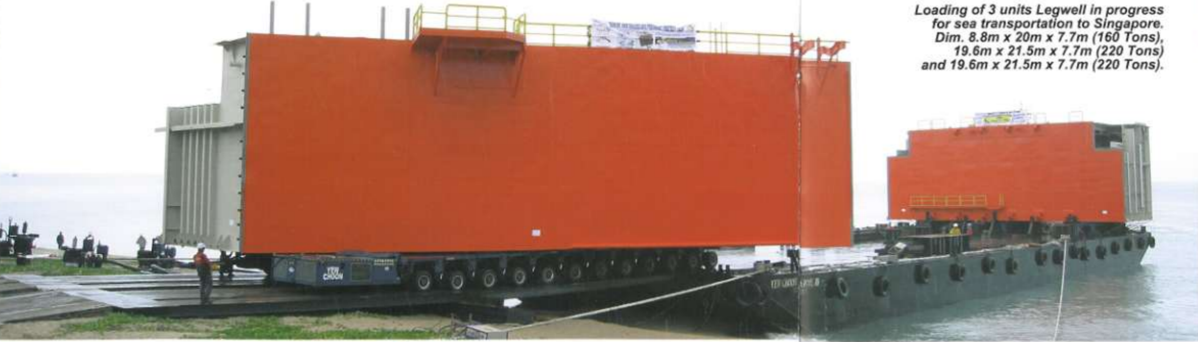
Load-in of second unit Block by ro-ro system. Dim. 26.5m x 21.5m x 7.6m (491 Tons).
