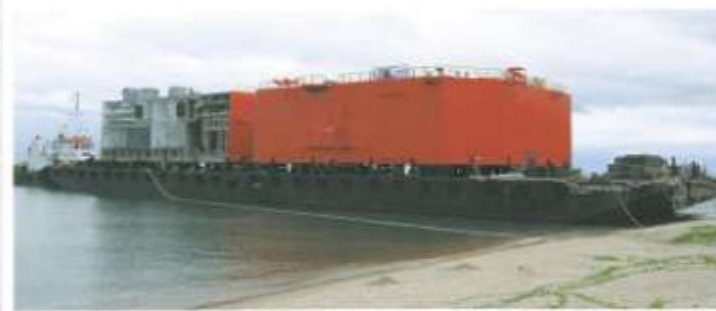
Loading of 3 units Legwell in progress for sea transportation to Singapore. Dim. 8.8m x 20m x 7.7m (160 Tons), 19.6m x 21.5m x 7.7m (220 Tons) and 19.6m x 21.5m x 7.7m (220 Tons).
