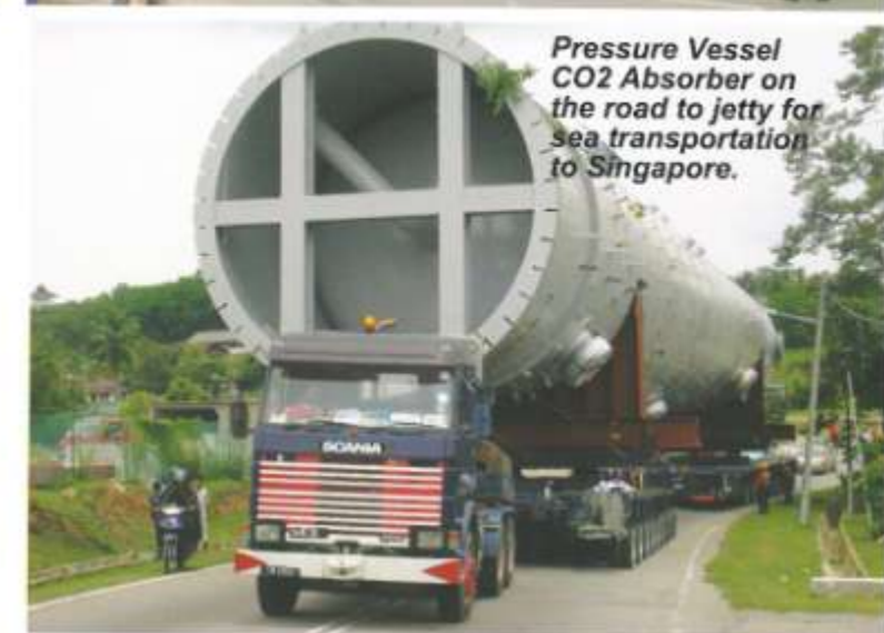
Arrival of Pressure Vessel CO2 Absorber for loading to barge. Dim. 51.8m x 6.54m x 7.66m (389.88 Tons).
