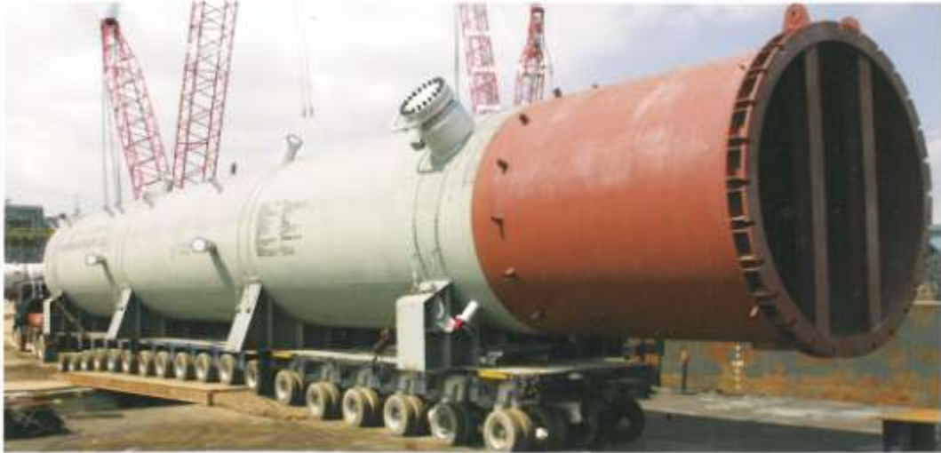
1 unit Reactor being transported by land to site. Dim. 35.06m x 5.03m x 5.1m (213 Tons).
