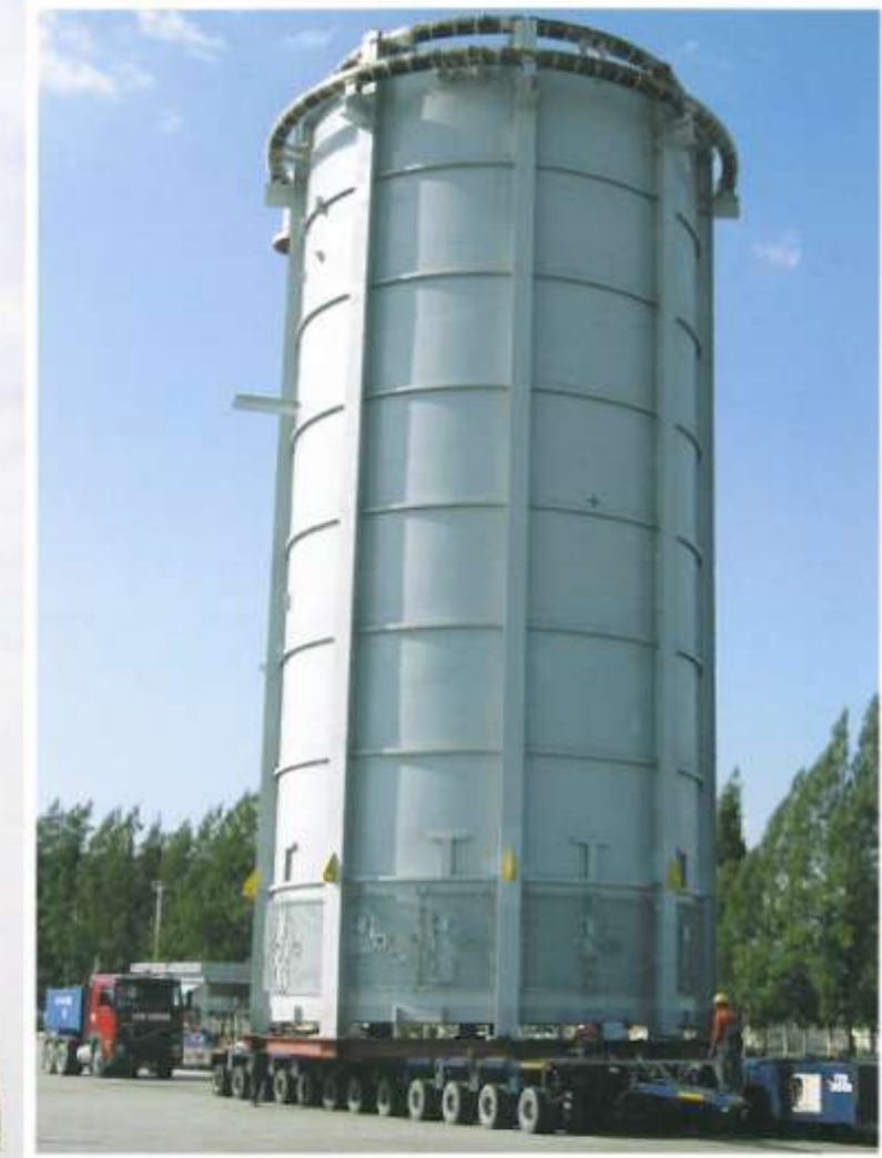
Land transportation of Heater, Dim. 7.5m x 150m x 79m (90 Tons).
