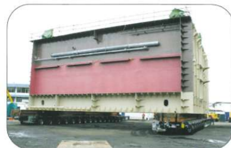
Singapore Load-on 650 tons heavy lift at UDL Shipyard.
