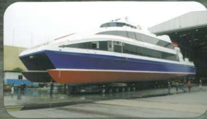
Vessel on hydraulic trailer.
