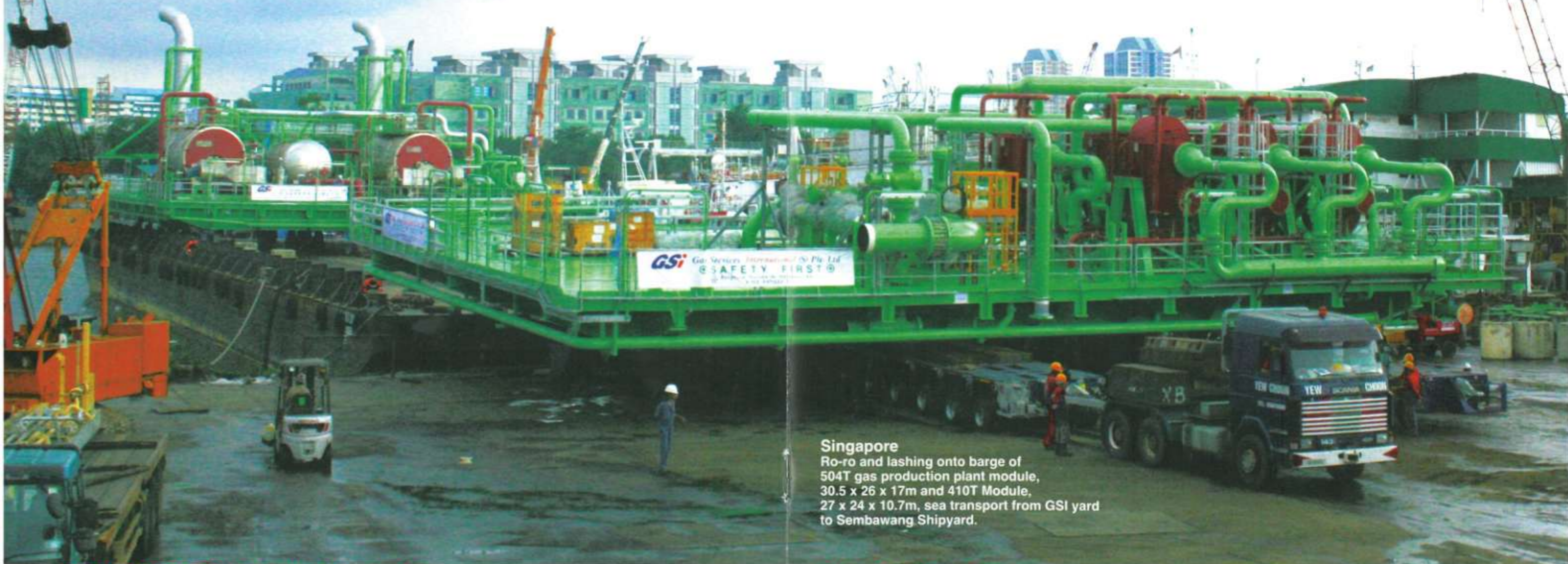
Singapore Yew Choon moved 14 units of these Modules and Structures from the storage area to the sea-front. The biggest is 850 tons, 29.5 x 19.3 x 12m.
