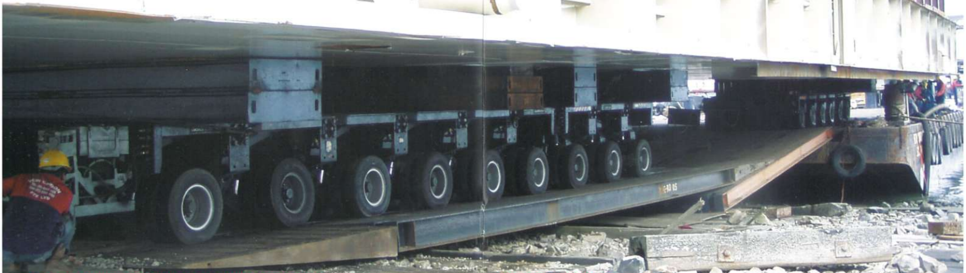
Load-on 420T Legwell and 420T Spudcan at Unithai Shipyard, Thailand.
