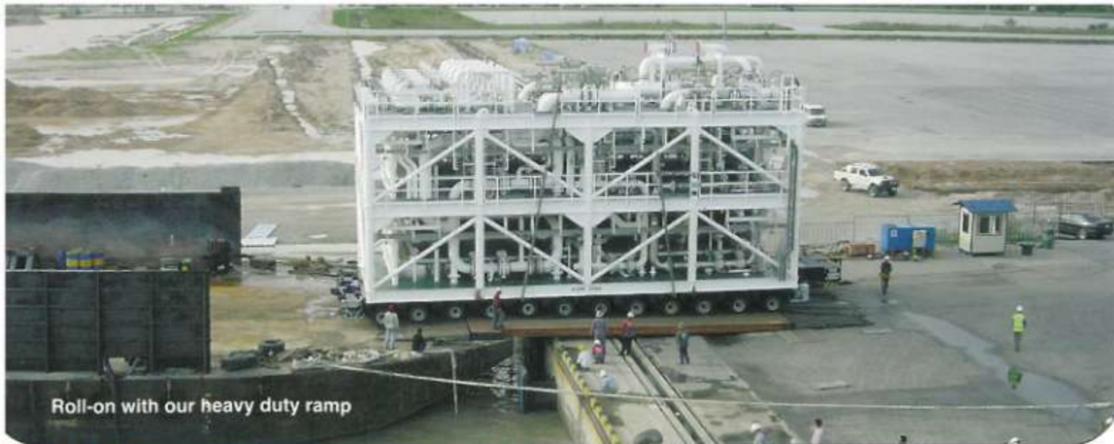
Transport by self-propelled trailer due to tight space constraint
