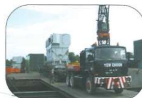
Offload from barge by ro-ro system with double ramp.
