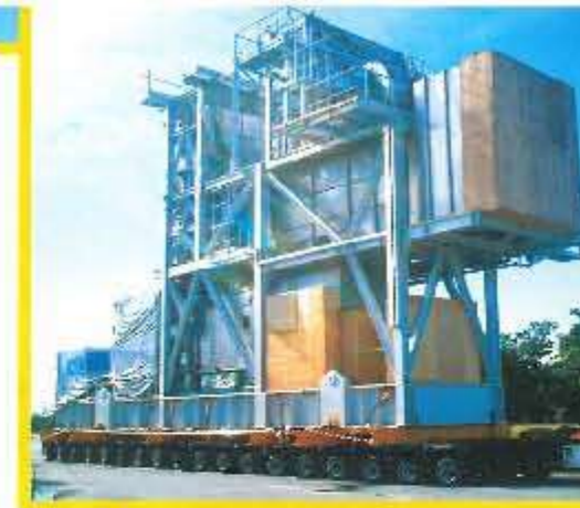
Goldhofer hydraulic trailer is used to transport this 18.5m high turbo heavy compressor by 18 axle lines, 1 1/2 configuration.
