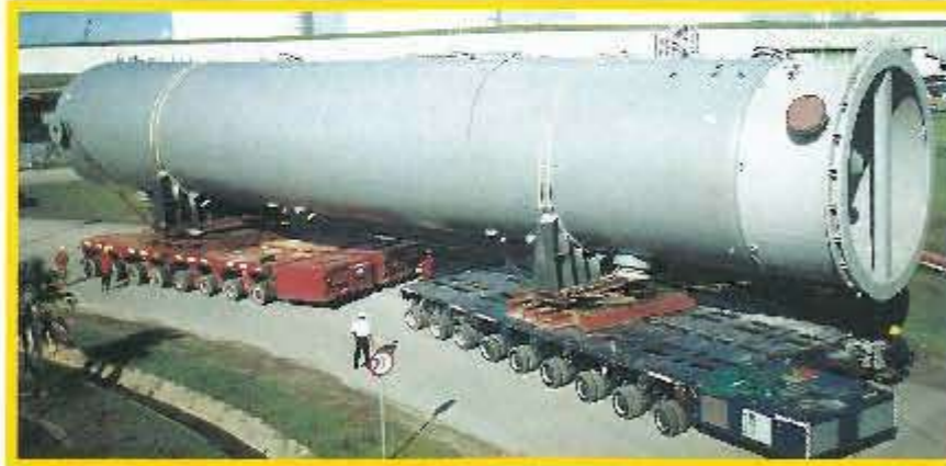
Land transportation of Heavylift by 2 units self-propelled trailer (spt).
