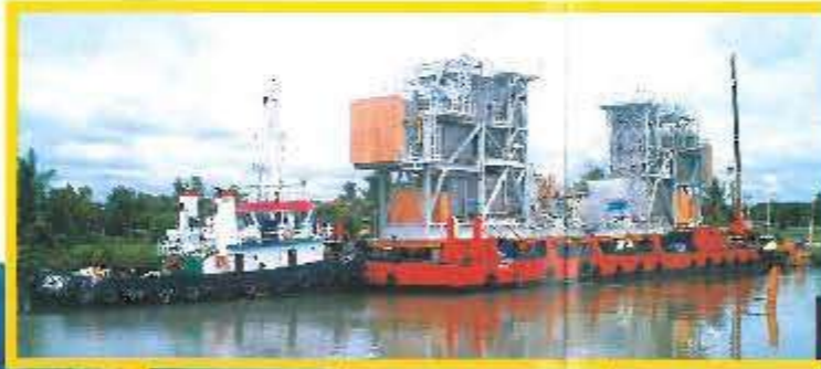
270 tons Turbo Compressors on the way to Senpah, Indonesia. Dimension of cargo: 27 x 7.3 x 15m.
