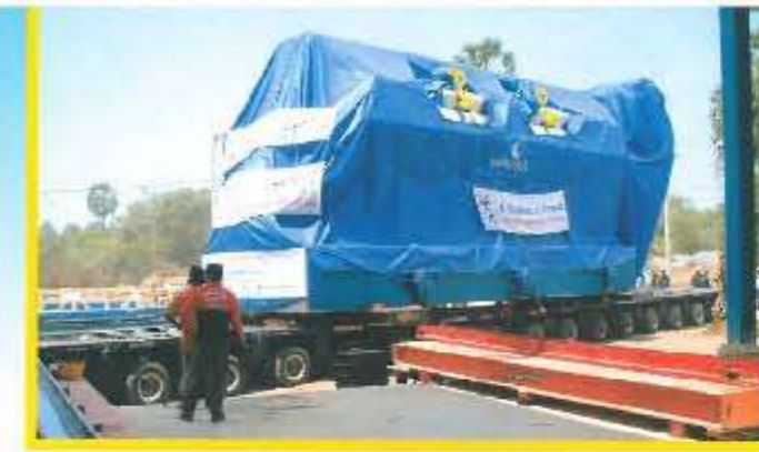
The skidding channel is positioned under the Engine. The hydraulic trailer jacks the Engine down onto the skidding channel.
